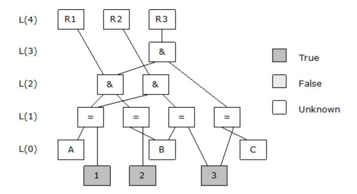
Within the internals of the NodeBrain interpreter you say that cell (A=1) has "subscribed" to changes in the value A, and that the cell ((A=1)&(B=2)) has subscribed to changes in the value of (A=1) and to the value of (B=2). Let's look at what happens when you make an assertion about A and B.
