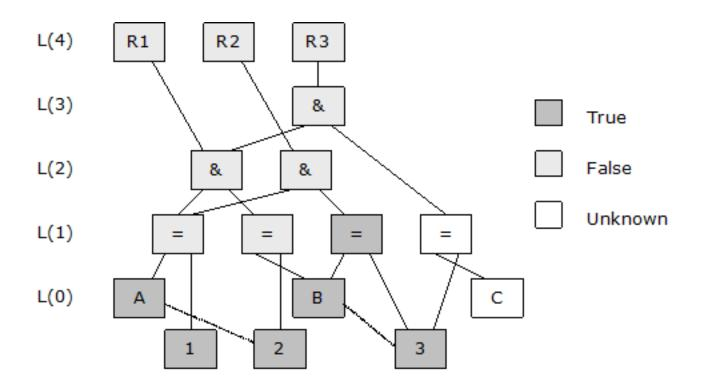
The impact of the changes to A and B are realized level by level. When A is assigned 2, this is a change, so A publishes a change to the (A=1) cell. This simply means (A=1) is scheduled for evaluation. When B is assigned 3, this is also a change, so B publishes a change to (B=2) and (B=3) because both have subscribed to changes in B.
