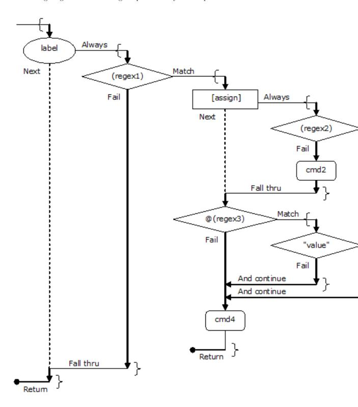
Translators are intended primarily as a way to uniquely identify a line of text and provide a single response. For this reason, the default behavior on a true condition is to execute the subordinate statement and terminate. A simple translator is just a series of patterns to match to the text buffer. The statement following the first matching pattern is executed and the translator stops.
